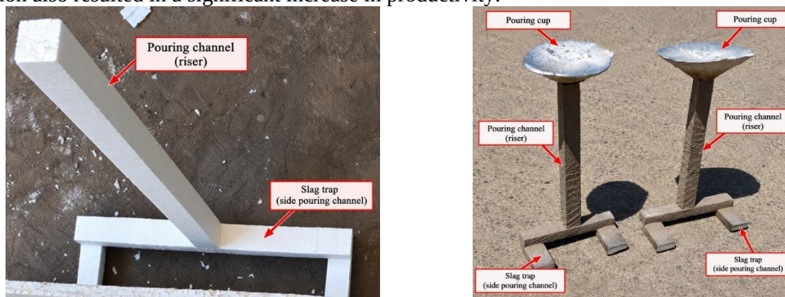
Figure 5. Pouring channel and feeders made from polystyrene material and cut from the finished patterns for casting gray cast iron alloy.
