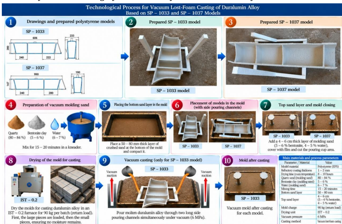
Figure 7. Integrated technological workflow for vacuum lost-foam casting of gray cast iron alloy using CNC-fabricated polystyrene patterns
